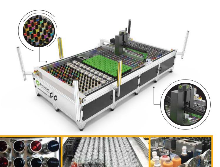
In advanced models, the recipe preparation process for solution bottles is done automatically via full automatic powder dyestuff weighing and solution preparation unit.
