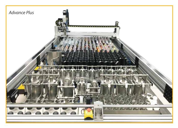
ENMOS laboratory dosing system has been developed for laboratory requirements within the scope of textile dyehouse solutions. The system is based on the principle of preparing multiple color solutions and is designed to support recipe trials for color matching the laboratory before actual dyeing recipes are given to batch dyeing.
