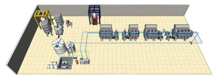
This system, which we call the ring system, is an advantageous system in long distances and in factories with high amounts of salt and soda. In this system, there should be two separate pipelines for salt dispensing and soda dispensing. The dissolved salt and soda is in continuous circulation in the pipelines.
